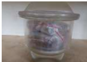
Fig 5.1(b): Keeping soil in Desiccator for maturity
