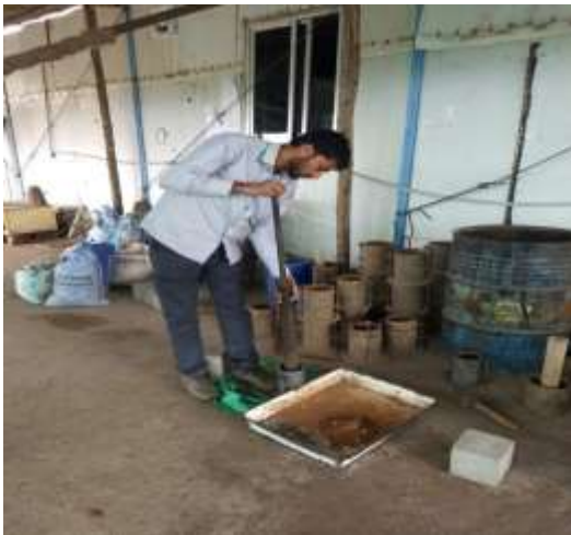
Fig 4.1.3: Conduction of Standard Proctor Test. 4.1.4 CALIFORNIA BEARING RATIO TEST: Test is conducted based on IS: 2720 Part(XVI) - 1965
